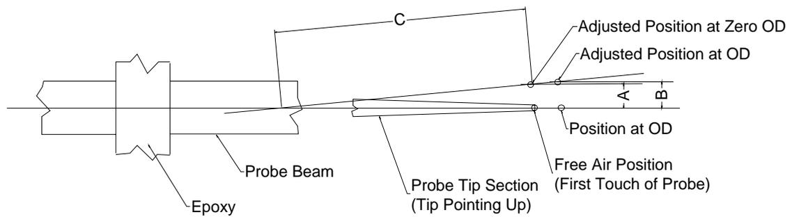
Probe Repair Position - Zero OD versus Overdriven Position
