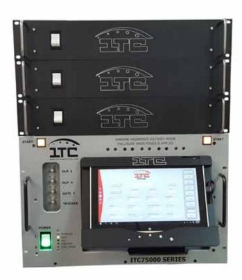
These additional tests require a processing unit containing a single board computer and digitizer, a logic controller for setting various test parameters, a High Voltage programmable clamp and a remote POD situated close to the device under test to provide gate drive, signal conditioning and the final stage of the clamp.
